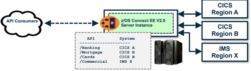
z/OS Connect EE V2.0 becomes the REST API entry point to the LPAR for access to several backend systems where the data program resides
